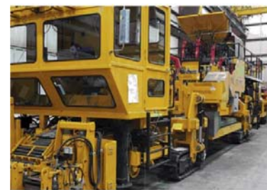
Tie Plate Distribution
