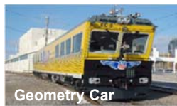
Semi Autonomous Track Inspections
